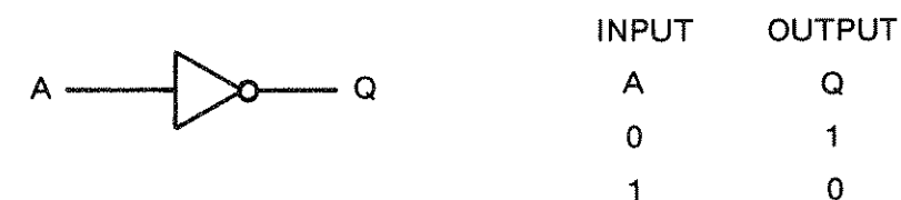
Figure 2.1 Inverter Diagram and Truth Table.
