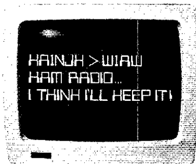
Fig 2—In monitor mode, your TNC responds to all of the packet activity on a frequency—even if the packets are not addressed to your station. Your computer displays the action.
